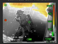
**Seamless operation.** No forced shuttering when transitioning between hotter and cooler areas of a scene.
